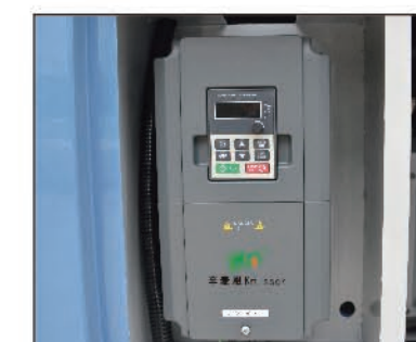
永磁驱动器 Permanent magnet motor is driven by inverter
